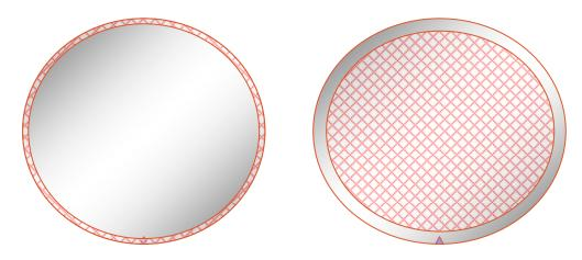
**Figure 1:** Cross-hatched areas show areas where VPD takes place. On the left, the edge can be analyzed by itself with automated VPD whereas on the right an inner area (or entire wafer) can be analyzed.
