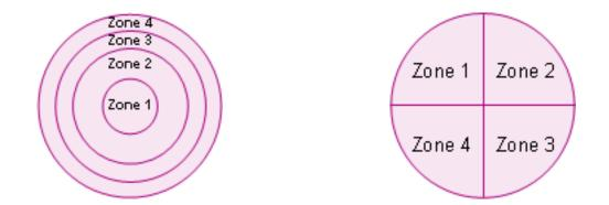
**Figure 2:** Automated VPD allows specific analysis of different zones, whether radial as in the wafer picture on the left or specific quadrants in the picture on the right. Contamination in certain areas can be traceable to specific tools or process points.
