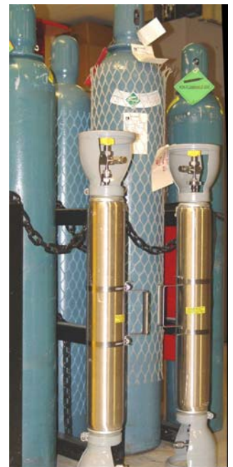
Inert gas cylinders and sample bombs for sample collection and inert gas analysis.
