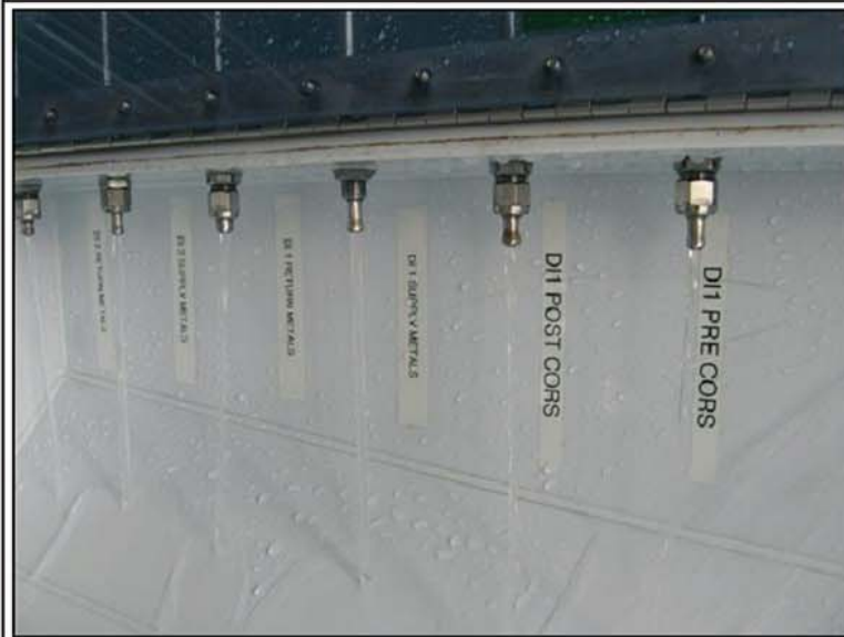
Figure 3. Close-up of sample lines under a Plexiglas cover.
