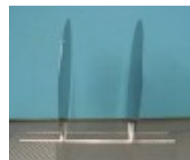
Figure 1. Specially prepared wafers for SMC monitoring
