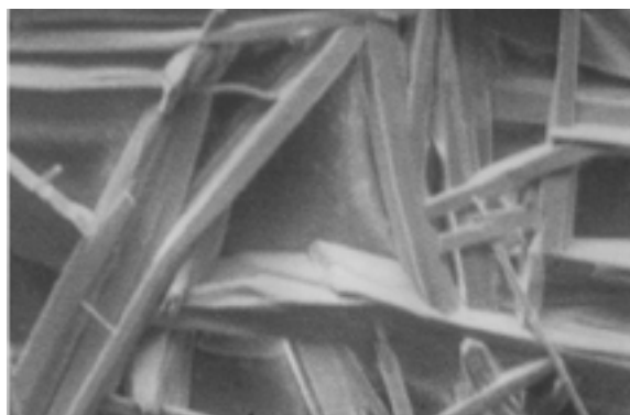
b) FRPP surface after interacting with UPW (magnification: 7.77 \times 10^3 )
