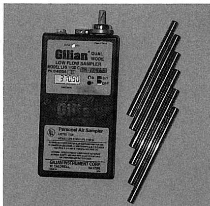
3. A typical organic air sample collection apparatus uses multiple media types to collect samples.
