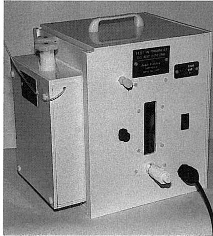
5. The typical collection period for inorganic air sampling devices is 24 to 72 hours.
