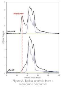
non-dispersive infrared detector (NDIR). The output of this analysis is a report containing the chromatogram (see Figure 2) and the spreadsheet providing organic speciation to the following content:
