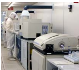
ICP-MS in Class 10 laboratory for water and chemical analyses
