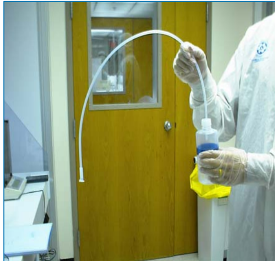
Figure 1: Ultrapure PFA Sampler. The sampler uses no o-rings or moving parts allowing for ultra-clean sample collection.
