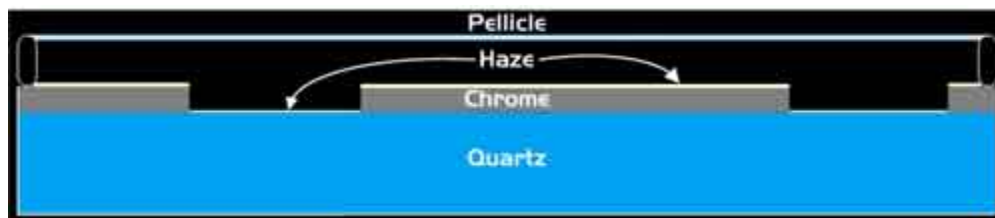
Representation of haze build-up occurring on a photomask
